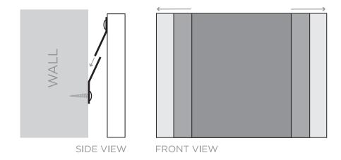
French cleats can also be used to fit corner Tri Trap panels. Remove plastic protective sheet from top and bottom of panel. Fix cleats as per previous instructions (1-3) on 2 sides.
