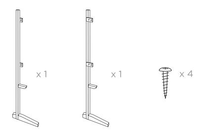
Place panel on its side. Position leg next to panel with foot facing towards front and support strut flush against bottom of panel. Screw in place using screws provided.
