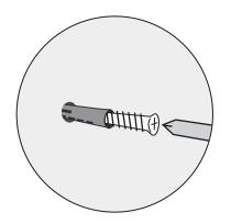
3 Slide panel down onto wall screws.
