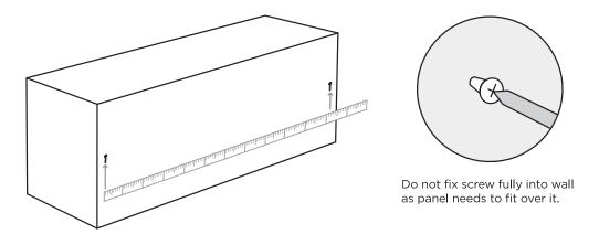
3 Push panel onto screws and pull downwards to secure into place.
