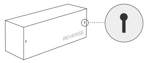
Measure width between centres of keyholes and mark on wall.
