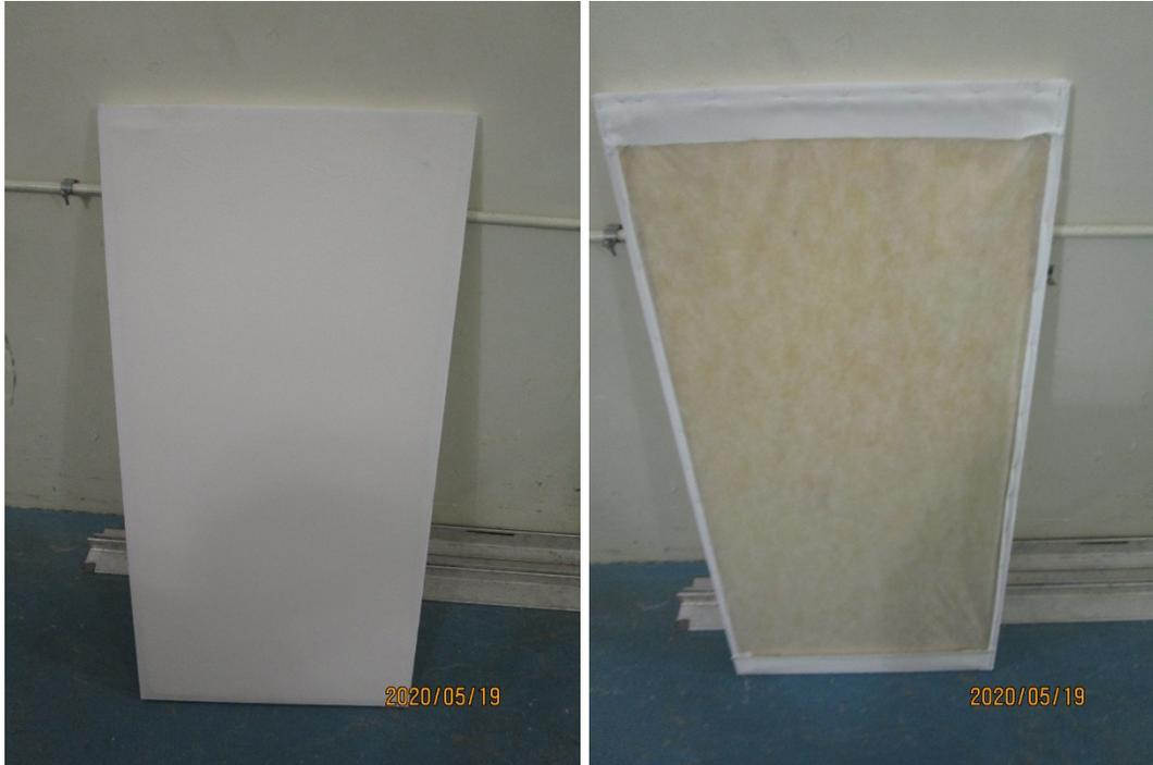
Figure 3 – Front (left) and rear (right) faces of individual specimen panel
